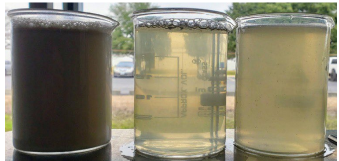
DAF Effluent: < 0.5% Feed Vol. as Waste L to R: Waste, Filtrate, Feed
