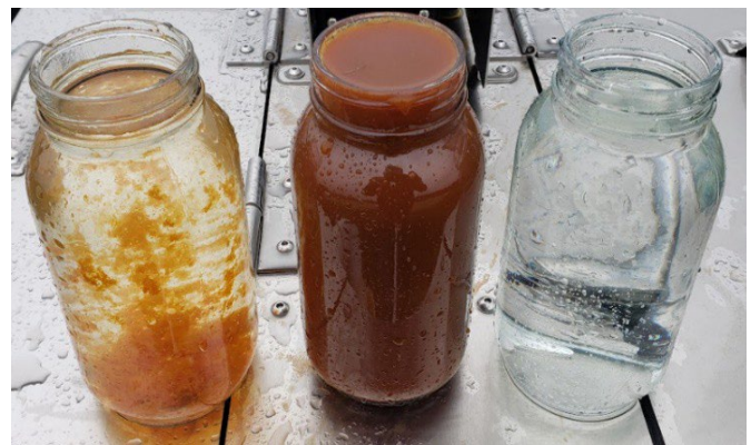
Total P Reduction: < 1.0% Vol. as Waste L to R: Feed, Waste, Filtrate
