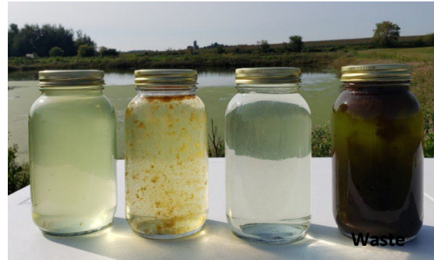
RAW WATER – Fe DOSED – FILTRATE – WASTE
